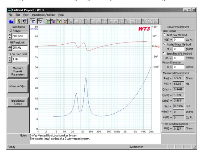
Here is a typical result when measuring a single full range driver in a vented box type enclosure:
